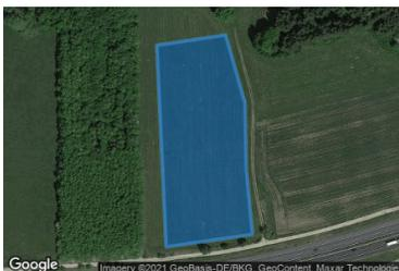
**Name:** PV Feld West**Axis tracking:** Fixed (no rotation)**Tilt:** 20.0 deg**Orientation:** 180.0 deg**Rated power:** -**Panel material:** Smooth glass without AR coating**Vary reflectivity with sun position?** Yes**Correlate slope error with surface type?** Yes**Slope error:** 6.55 mrad**Approx. area:** 37,276 sq-m
