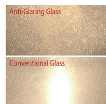
Using high quality and low reflective glass, reduce the typical direct light reflection of about 10% on conventional glass down to less than 3%. Especially in sensitive utility project locations like airports, highways along railways or for noise reductions walls. Avoids costs for counter measurements of blending solar modules.
